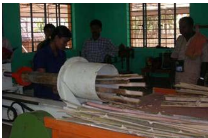
Trainee at work on a bamboo splitter at Don Bosco Training Centre
